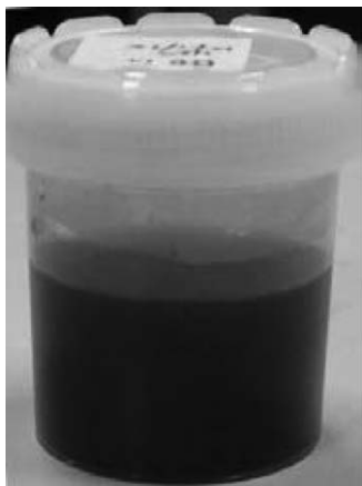
Figure 3. GO suspension in distilled water obtained by bath-sonication.
